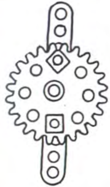
Fastening Strips to Pierced Gear
