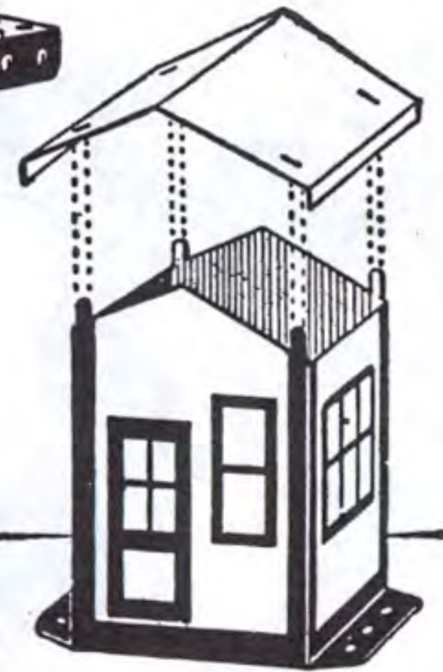
Method of Assembly of Roof to House
