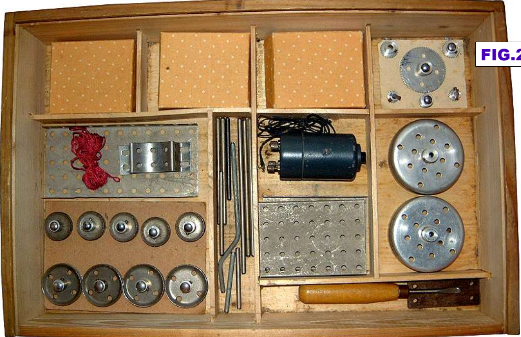
FIG.1 wide Screwdriver is needed for the Grubs in the Collar. Also in the Set, some parts not in the Manual and perhaps not original: 51mm Ø black Rubber Rings on the 36mm Pulleys, and 3 Axle Stops which look exactly like MÄRKLIN #35a.
