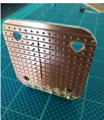
9. Insert the IC socket and mark where to cut the track. Don't cut the tracks for ground (4,5,12,13) like I did!
