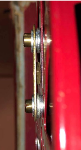
Peter Sullivan in Switzerland came up with this great idea to hold the firebox door closed. A nut is held captive behind a 3-hole Strip.
