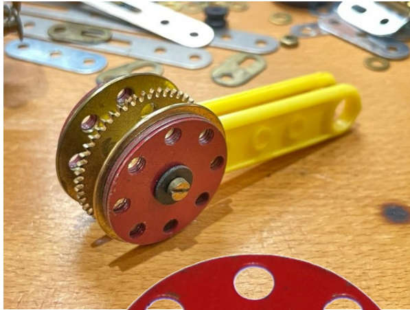
Peter Sullivan in Switzerland came up with this great idea to hold the firebox door closed. A nut is held captive behind a 3-hole Strip.
