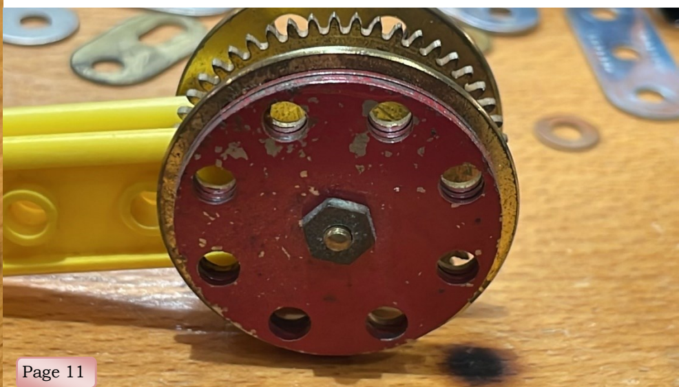
From Tim Gant is this neat idea to make an insulated train wheel using a 24a Wheel Disc as the flange with the smaller 217a Wheel Discs as the 'tread'. An Elektron 6ba Bolt and an Elektron Insulating Bush acts as the axle and keeps the wheels insulated from each other. The 50t gear is pre-1912 to ensure the wheels are close enough together to run on 00-gauge track. This lone axle was built purely to illustrate that it was possible to create a driven axle of a Hornby type train (taking its power from the rails) without butchering parts. My first version in that working engine used Army Multikit shells which I had threaded 5/32 BSW at each end. The drive was via a pulley (ca. 1910) which I found was a tight fit on some of the shells; however, over time the drive band perished, and it would be a pain to replace.
