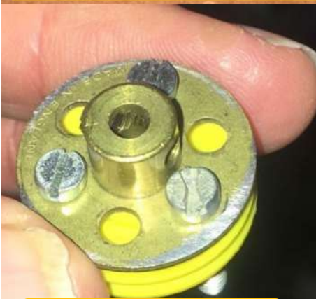
Bolt an Elektrikit part 518 to a part 22p Plastic Pulley with boss. If you use a 1" Bush Wheel from the DBDY Road Wheel set, you will need washers to allow for the peening ridge.
