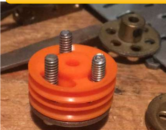
Bolt an Elektrikit 1" Bush Wheel part 518 to 1" Plastic Pulleys without boss part 22bp.
