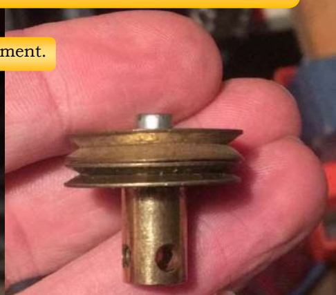
Bolt part 22a Pulleys without boss to a part 64a Short Threaded Coupling.
