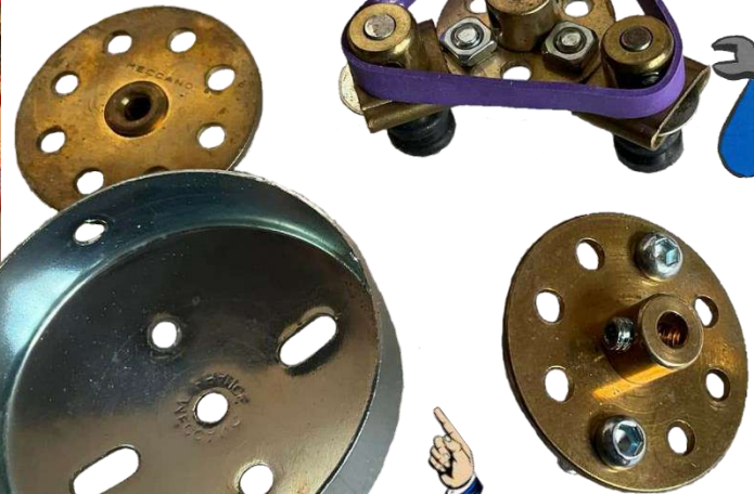
Fig 1. I've used a part 162a Boiler End as the drum. Long Bolts are fixed to the part 24 Bush Wheel then journaled through the Boiler End and into the holes in the outside Bush Wheel thus sandwiching the Boiler End in-between the Bush Wheels.
