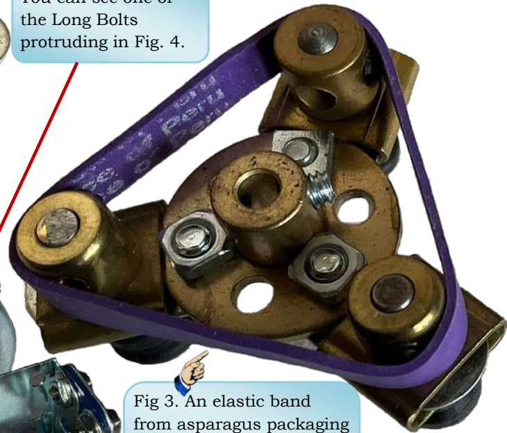
Fig 1. I've used a part 162a Boiler End as the drum. Long Bolts are fixed to the part 24 Bush Wheel then journaled through the Boiler End and into the holes in the outside Bush Wheel thus sandwiching the Boiler End in-between the Bush Wheels.
