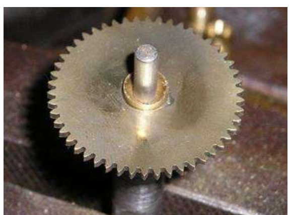
Spur gear with the boss inserted
