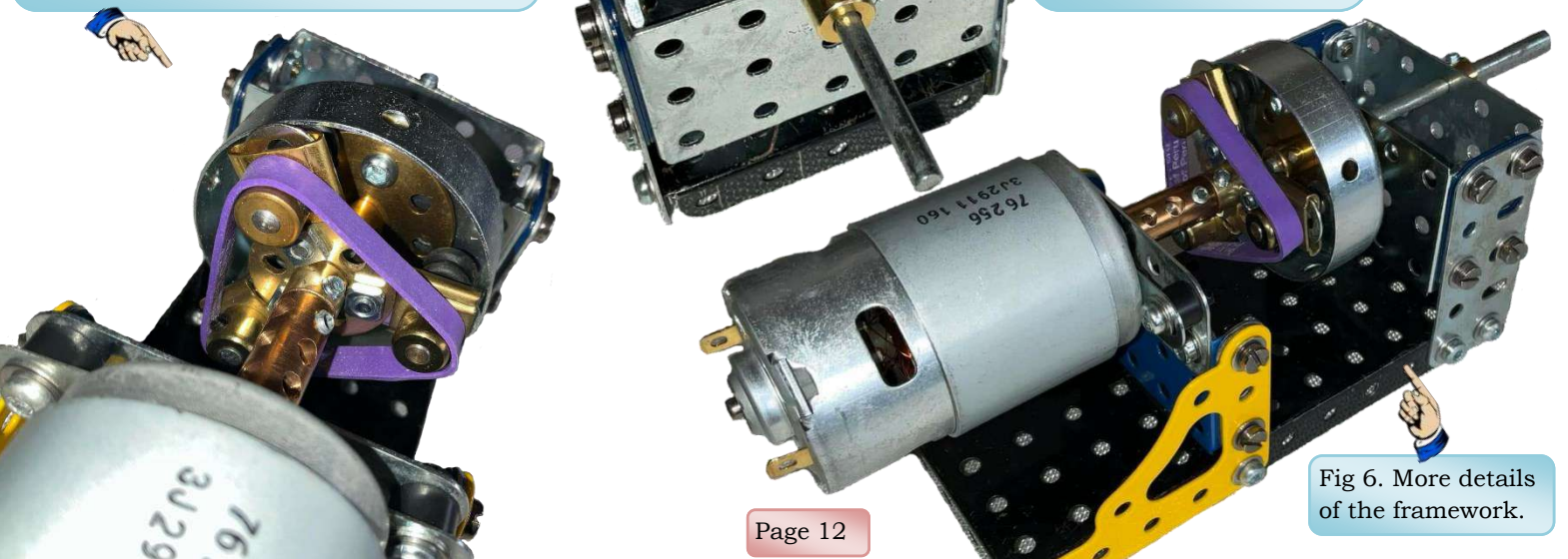
Fig 3. An elastic band from asparagus packaging is used to keep the Rubber Pulleys retracted at slow speeds.
