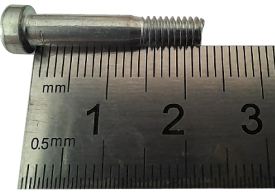
147g (A347) - Pivot Bolt, 23 mm (29/32"), hex socket head
