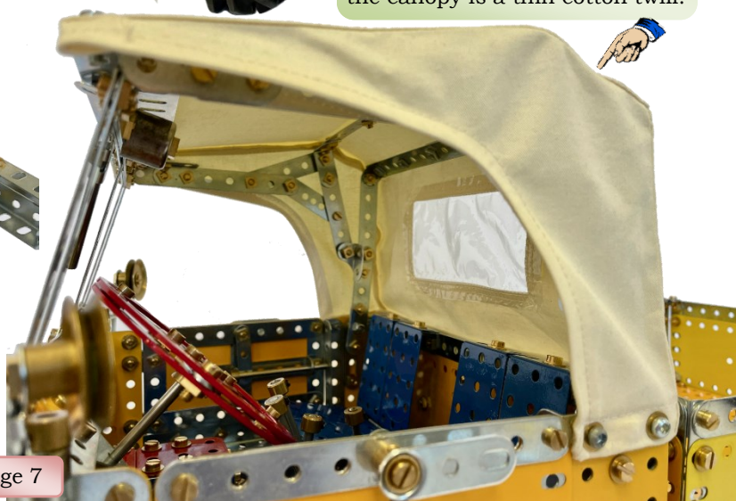
Fig. 12. The hood struts seen from the inside. The fabric of the canopy is a thin cotton twill.
