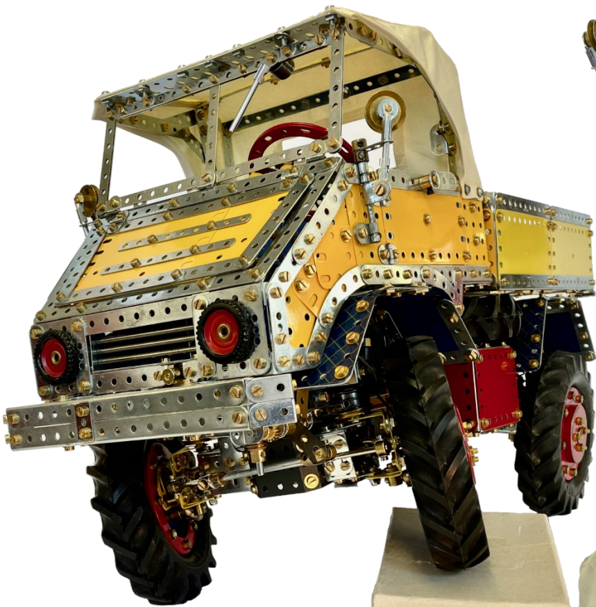
Fig. 10. Demonstration of the axle articulation in practice.
