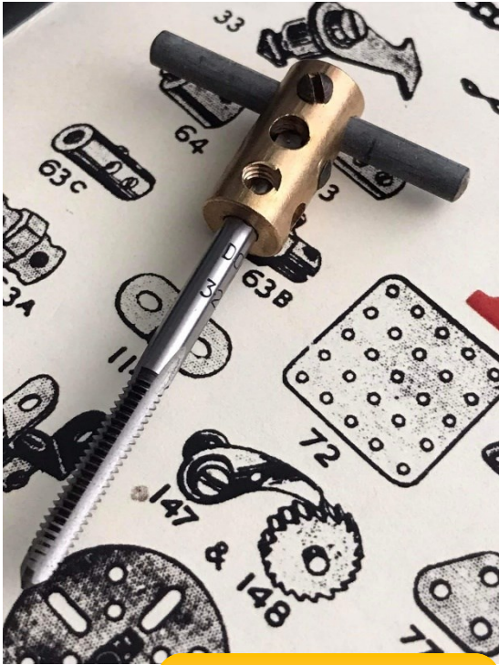
From Danny Skyrme. Clean out your threaded holes and debur threads in bosses with this neat little tap holder.
