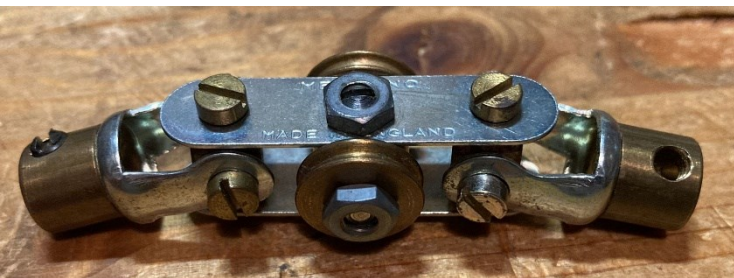
Solution: Add an early half inch pulley secured either side of the narrow strips. Hold in place with a pivot bolt through the plain hole of the collar. The narrow strips are attached to the collar with long grub screws and a flat nut. An Elektrikit washer is placed under one of the narrow strips.
