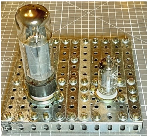
The proof-of-concept chassis with octal and B9A valve bases
