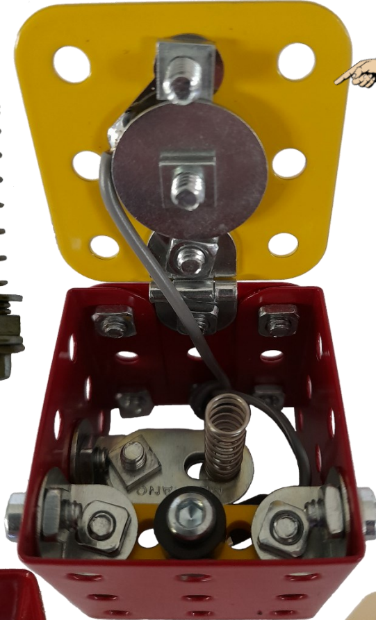
From Tim Gant. Mounting an N20 motor using only standard parts. No filing or drilling. Yet again we find that Frank Hornby had all the answers without going off into the wilderness.
