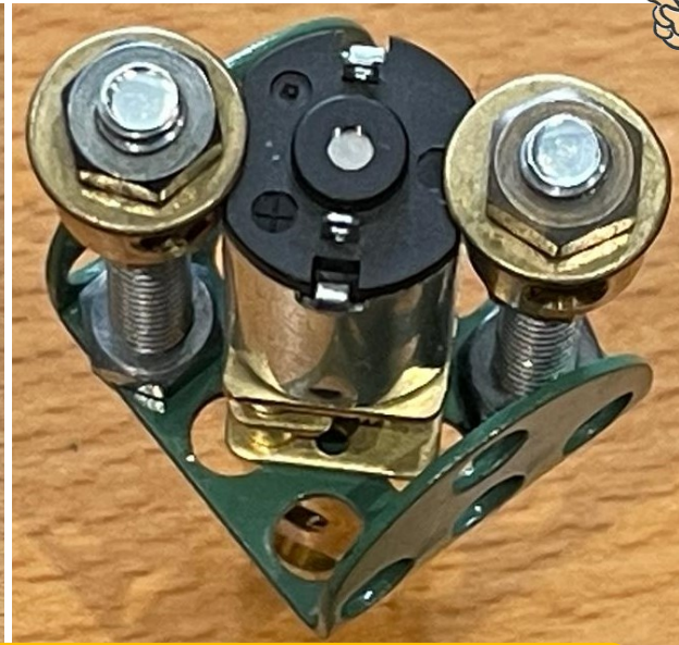
From Tim Gant. Mounting an N20 motor using only standard parts. No filing or drilling. Yet again we find that Frank Hornby had all the answers without going off into the wilderness.
