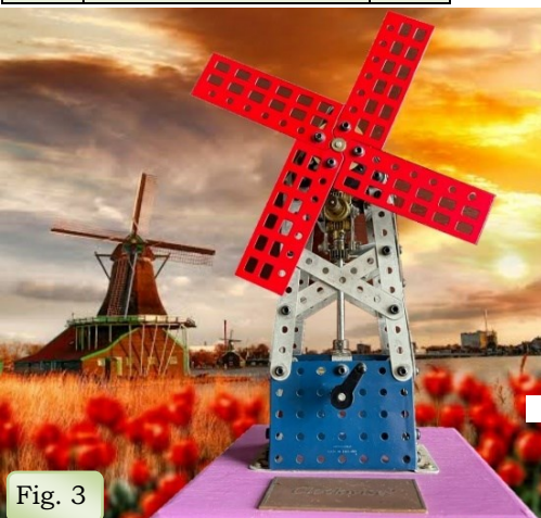
Fig.3 Tomkinson-Denny constant-direction drive in all its amazing complexity! A Pawl attached to the frame of the windmill engages the 19t Pinion at the bottom end but was forgotten by the photographer.
