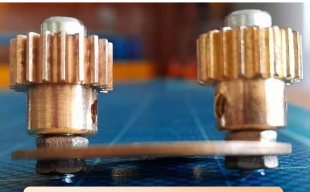
Step 1. Bolt Pinions to Wheel Disc using BC2 method making sure they spin freely.
