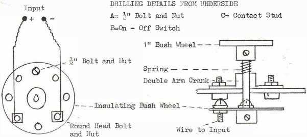
The control box features a single reversing switch serving four independent on/off switches for each crane motion. The board is made from any suitable insulating material (eg. Formica) cut to fix to a suitable box. The wire used is bare copper and soldered joints are recommended.
