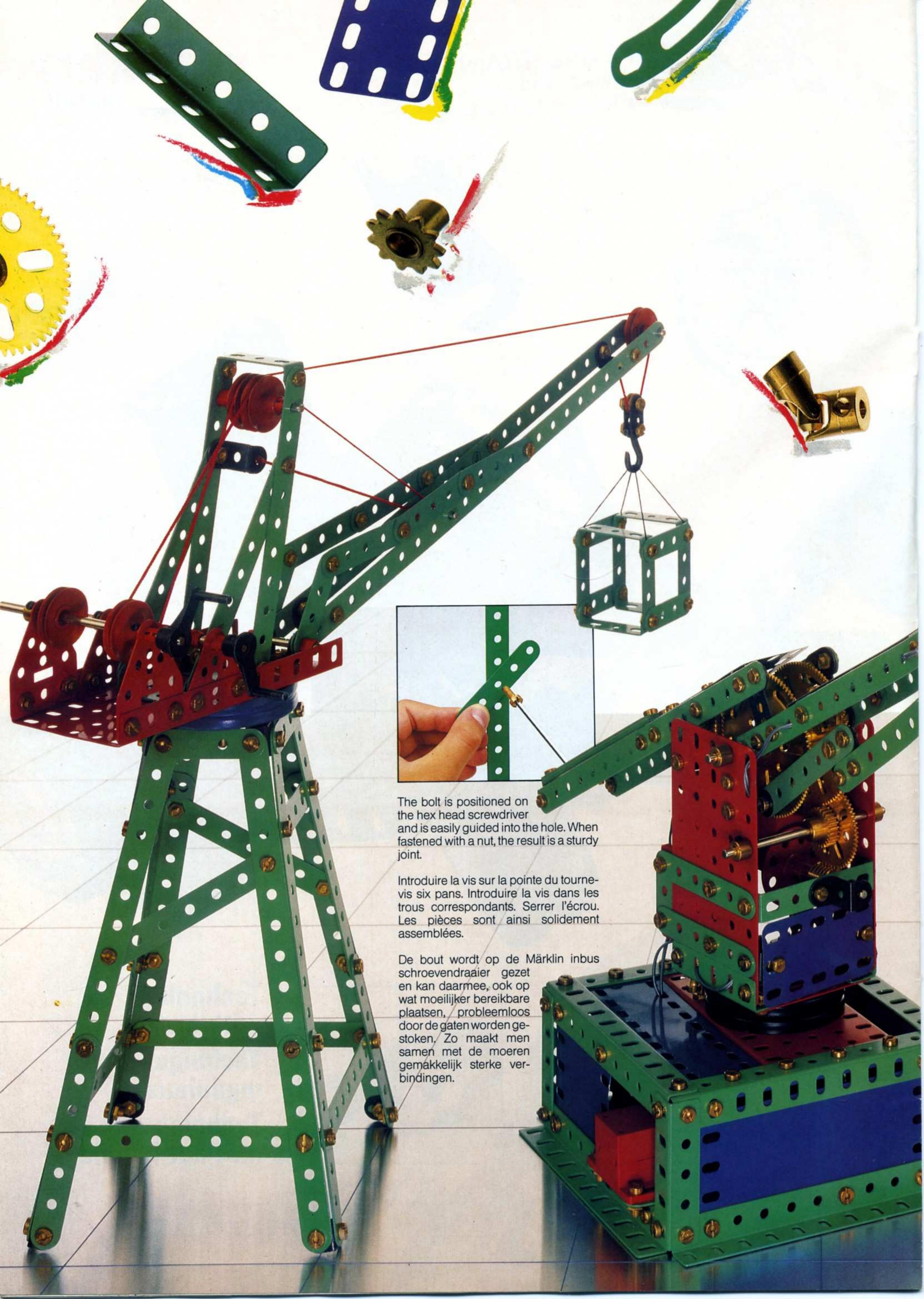
The bolt is positioned on the hex head screwdriver and is easily guided into the hole. When fastened with a nut, the result is a sturdy joint.
