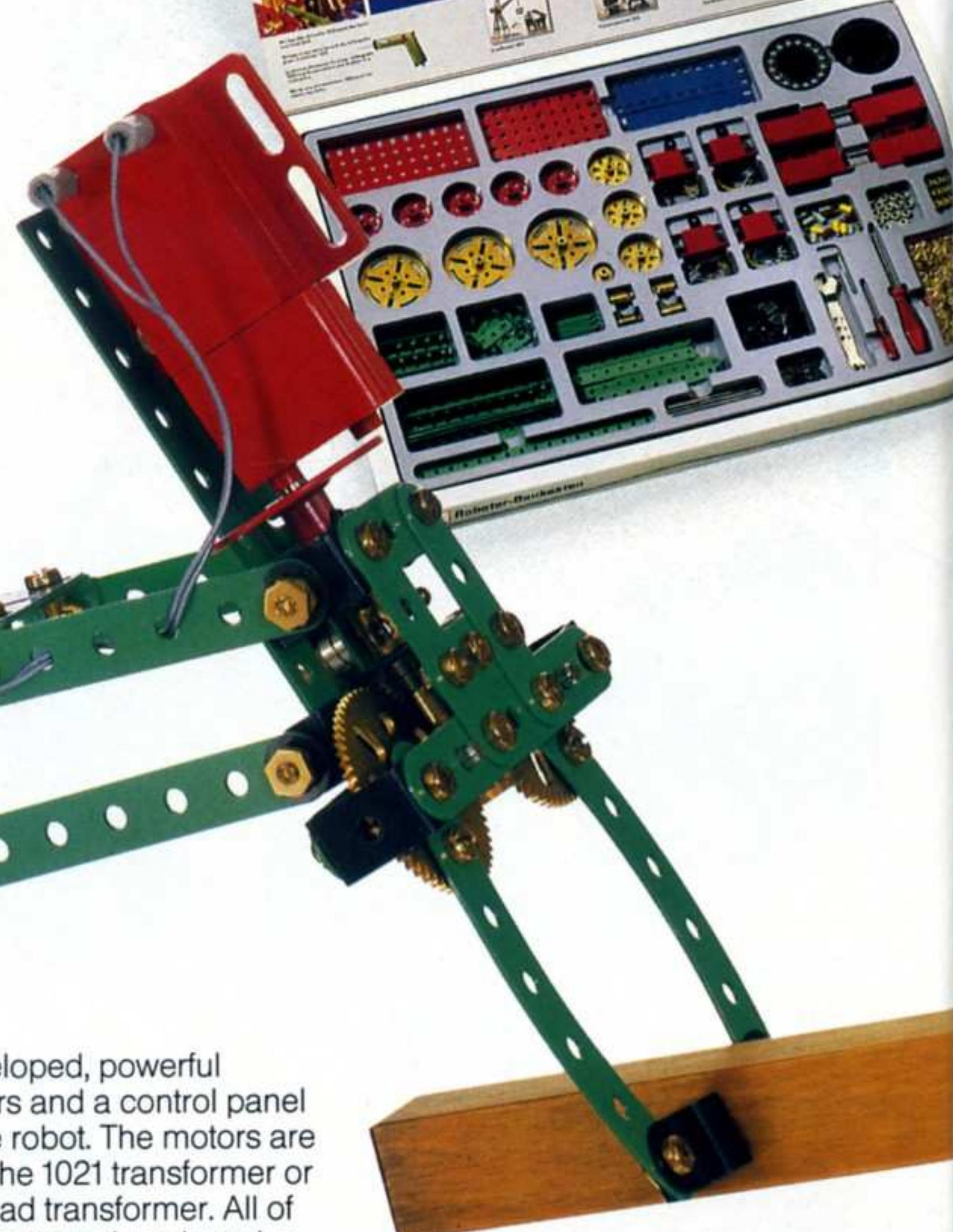
Four newly developed, powerful motors with gears and a control panel for operating the robot. The motors are powered using the 1021 transformer or any model railroad transformer. All of the motors are protected against electrical overload: motor burnout due to jamming is not possible.
