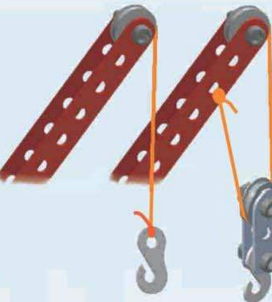
**USA** Simple and double arrangement of a string on a pulley wheel.
