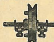
EC 38 Loose V Pulley. Secured by adjustable U pieces
